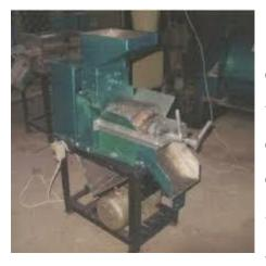
The machine is composed of a hopper, extracting chamber, stand/frame, the transmission, and the prime mover with 1.5 hp electric motor. This machine had an average extracting capacity of 50-60 kg/hr for whole and chopped rhizomes and 100 kg/hr for grated rhizomes. The overall extracting
