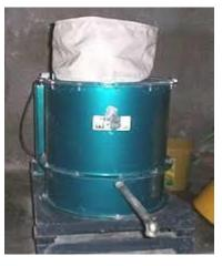
This machine is used to remove the excess water from the washed starch. Reduction in the water content of starch decreases the time of drying by 4 hours. It has a capacity of 12 kg per 12 min of centrifugation of the dripping wet starch. The
